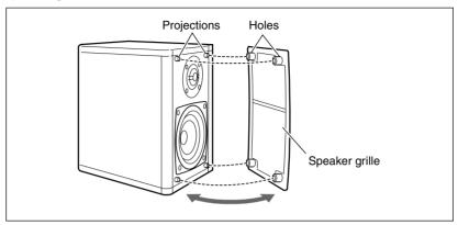
**To remove the speaker grille,** insert your fingers at the top of the speaker grille, then pull towards you. Repeat the procedure at the bottom of the speaker grille.
